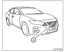
The AEB system uses a radar sensor (A) located on the front of the vehicle to measure the distance to the vehicle ahead in the same lane
