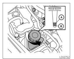
Check the fluid level in the reservoir
