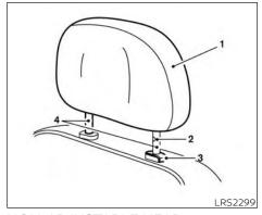
NON-ADJUSTABLE HEAD RESTRAINT/HEADREST COMPONENTS
