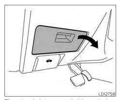
The extended storage switch is used when the vehicle is in transit from the factory. It is located in the fuse panel to the left of the steering wheel on the instrument panel. If any electrical equipment does not operate, ensure the extended storage switch is pushed fully in place, as shown.
