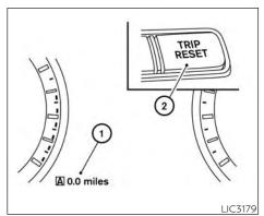
Odometer/Twin trip odometer
