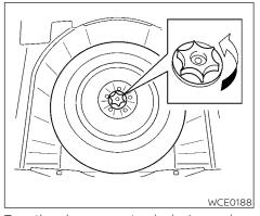
Turn the clamp counterclockwise and remove it to access the spare tire.
