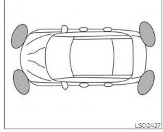
The sonar (parking sensor) system sounds a tone to inform the driver of obstacles near the bumper.
