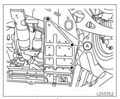
**Under-engine protector** Removal of engine protectors
