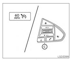
To set cruising speed, accelerate your vehicle to the desired speed, push the SET- (C) switch and release it. (The color of the cruise indicator changes to green and set vehicle speed indicator comes on.) Take your foot off the accelerator pedal. Your vehicle will maintain the set speed.
