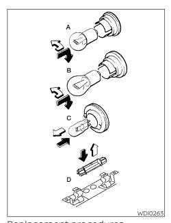
Replacement procedures All other lights are either type A, B, C or D. When replacing a bulb, first remove the lens, lamp and/or cover.
