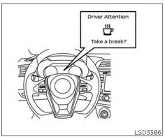
The system resets and starts reassessing driving style and steering behavior when the ignition switch is cycled from ON to OFF and back on.
