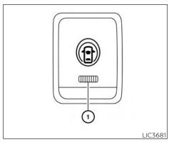
The dynamic driver assistance switch is used to temporarily activate the Intelligent Lane Intervention (I-LI) system that is enabled using the settings menu of the vehicle information display.
